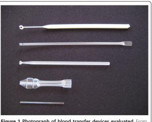
Figure 1 Photograph of blood transfer devices evaluated. From top to bottom, the loop, straw-pipette, inverted cup, calibrated pipette, and glass capillary.
