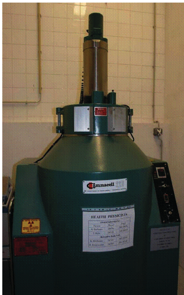
Figure 1 Cobalt 60 irradiator. The Gammacell 220 ® (MDS Nordion, Ottawa, Canada), an example of a conventional self-shielded irradiator. In the irradiate position the sample chamber is surrounded by several rods or "pencils" of the isotope. The dose rate of the cell is determined by the activity of the source, and the absorbed dose delivered to the insects controlled by adjusting the exposure time. The sample chamber is a vertical cylinder, approximately 150 mm diameter by 200 mm tall (3.7 L) and has a typical dose uniformity ratio of about 1.7. Such self-shielded isotopic irradiators ( ^{60}\text{Co} or less commonly ^{137}\text{Cs} ) are the main means of insect sterilization for SIT programmes worldwide.
