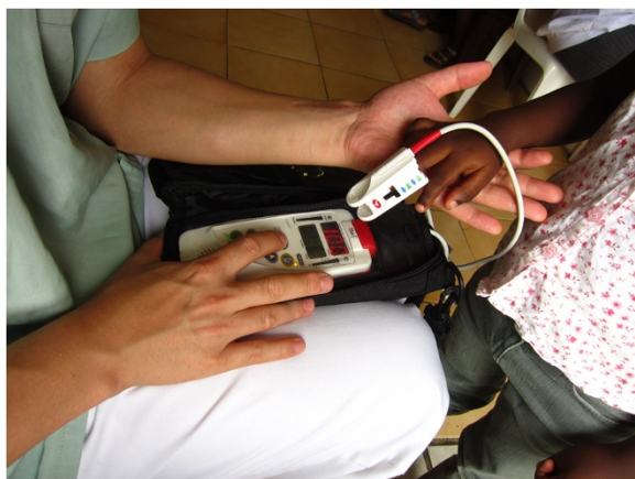
Figure 1 Methaemoglobin measurement with the pulse oximeter. RAD-57™ "Rainbow"® Pulse oximeter (Masimo) with fingerprobe for MetHb detection applied to the third finger of the right hand of a child (healthy control) during measurement. The finger/hand is held to reduce movement for 45–60 seconds and the procedure is non-invasive and painless.
