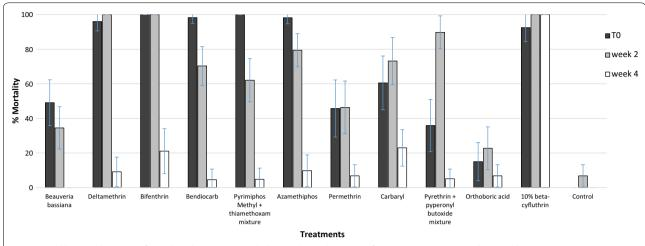
**Fig. 2** Weekly mortality rates of pyrethroid resistant *Anopheles gambiae* M'bé strain after exposure to insecticide treated insert using 3 min eave tube assay. Error bars indicate the confidence intervals for the different proportions on the graphs
