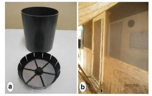
**Fig. 1** a Photo of the components of the eave tube assay; **b** Picture of the experimental hut fitted with eave tubes
