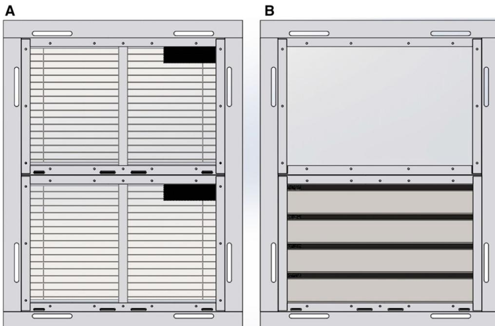
**Fig. 2** Prototype windows (internal view). Where **A** is the blinds window and **B** is a window combining a translucent panel at the top of the concertina panel at the bottom. Source: Jawara et al. [7]
