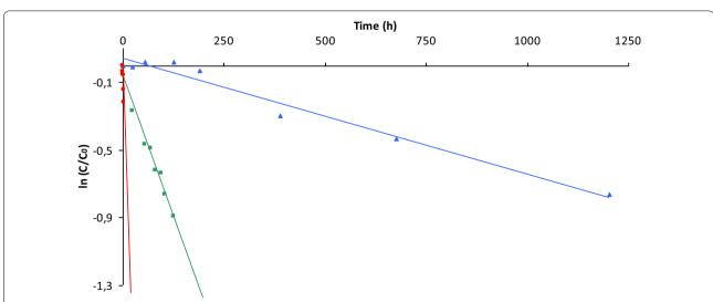
Fig. 3 First-order plots showing the degradation of artesunate (0.3 M phosphate, pH 9, 0.22 mmol/mL mannitol) at various temperatures: (filled circle) 313.15 k, (filled rectangle) 298.15 k, (filled triangle) 278.15 k
