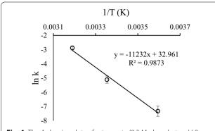
**Fig. 4** The Arrhenius plots of artesunate (0.3 M phosphate, pH 9, 0.22 mmol/mL mannitol)
