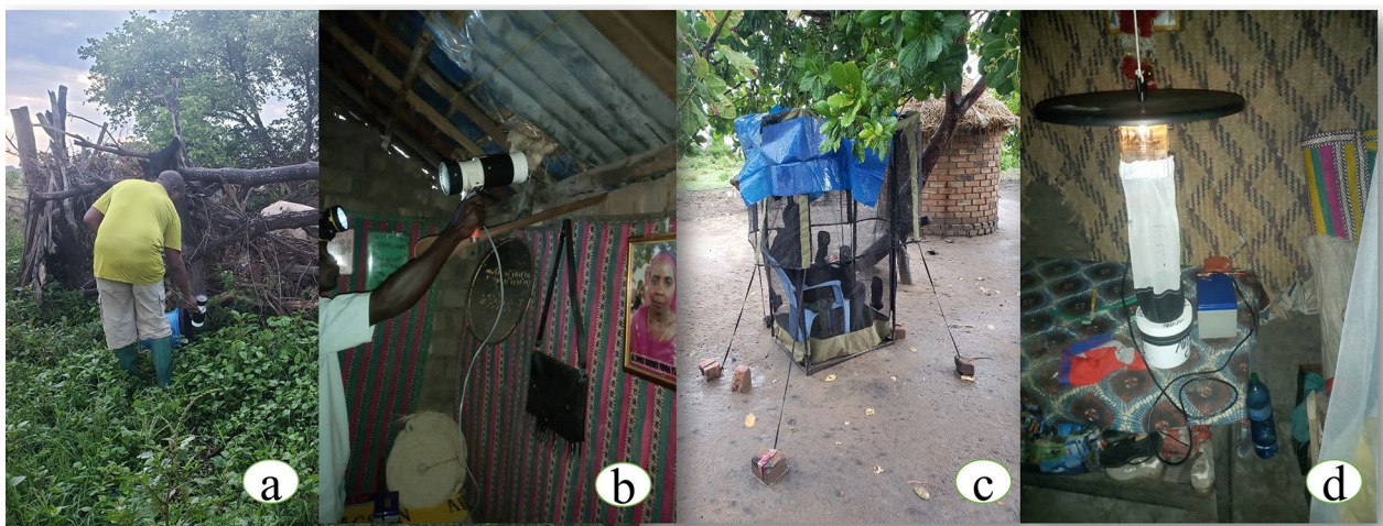
Fig. 3 Mosquito traps which were used for mosquito collections; a person collecting resting mosquitoes from resting bucket using prokopack aspirator near cattle shed (b) a volunteer collecting resting mosquitoes indoors using a prokopack aspirator (c) a double net trap (d) a CDC-light trap
