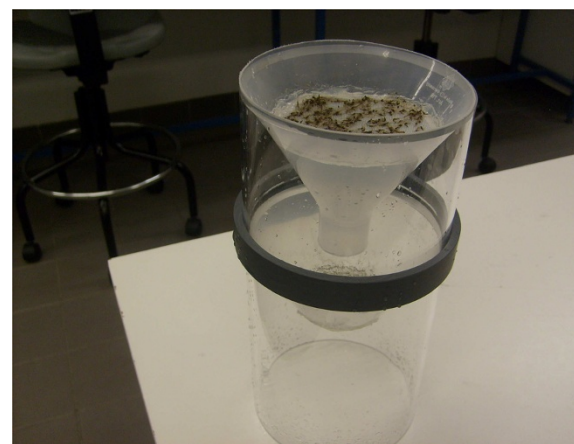
Figure 1 Apparatus for cleaning and drying eggs. Detachable funnels and rings holding the funnels above each other.
