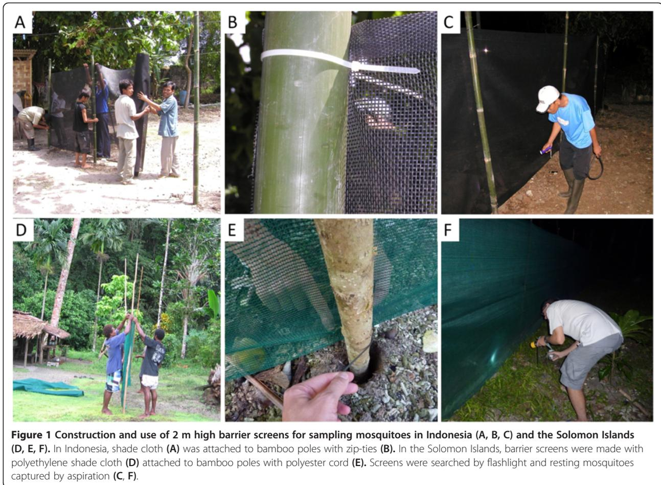
**Figure 1 Construction and use of 2 m high barrier screens for sampling mosquitoes in Indonesia (A, B, C) and the Solomon Islands (D, E, F).** In Indonesia, shade cloth (A) was attached to bamboo poles with zip-ties (B). In the Solomon Islands, barrier screens were made with polyethylene shade cloth (D) attached to bamboo poles with polyester cord (E). Screens were searched by flashlight and resting mosquitoes captured by aspiration (C, F).
