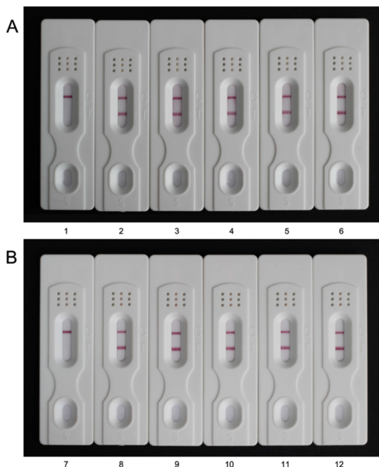
Figure 7 Dipstick specificity tests of commonly used anti-malarial drugs (A and B). Each standard solution ( 1 \text{ mg mL}^{-1} ) was diluted in distilled water at a concentration of 5,000 \text{ ng mL}^{-1} . (1) artemisinin; (2) quinine; (3) chloroquine diphosphate salt; (4) primaquine phosphate; (5) pyrimethamin; (6) blank; (7) artemisinin; (8) lumefantrine; (9) amodiaquine; (10) piperazine tetraphosphate tetrahydrate; (11) pyronaridine tetraphosphate and (12) blank. Each sample was analyzed in triplicates and the figure shows the representative pictures.
