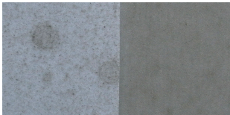
Figure 7 Spore distribution. Photo of a piece of proofing paper surface sprayed (left) or coated (right) with fungus formulation (zoomed in 4 \times ). Equal volumes of a 5 \times 10^9 spores/ml formulation (20% Ondina/80% Shellsol) were applied per surface area using the spray method described by Bell et al [35] or the optimized coating method. Spots on the left piece represent the spray droplets. The white background is not visible on the coated piece (right) because it is covered fully with the spore layer.
