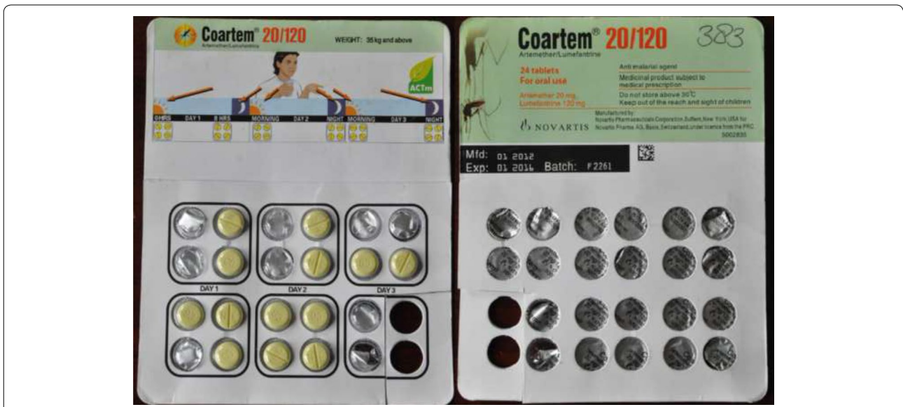
Figure 2 The suspect Coartem ® sample, having failed semi-quantitative thin-layer chromatography.
