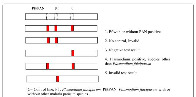
**Fig. 1** Test line configuration for HRPII based RDTs used in our assessments and their interpretation. Line configurations differed slightly depending on target antigen. In this study target antigens for RDTs included *Plasmodium* LDH, HRP2 and aldolase. Invalid test cassettes were noted and replaced during the assessments. *C*: Control line, *Pf*: *Plasmodium falciparum*, *Pf* + *PAN*: *Plasmodium falciparum* with or without other malaria parasite species
