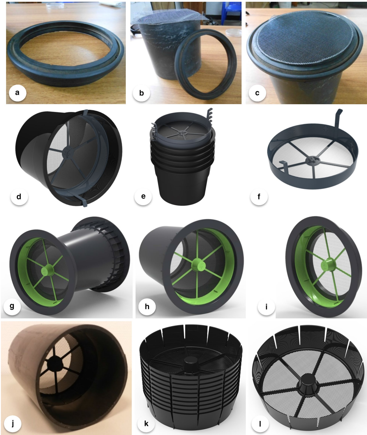
Fig. 2 Eave tube prototypes. Originally, electrostatic netting was fitted over the PVC pipe using a rubber or PVC ring (a–c). Subsequently a second generation of tubes with special inserts (d–f and g–i) was developed. Unfortunately these inserts were too close to the outside of the house, which resulted in the development of an eave tube insert that can slide inside the PVC pipe (j), can easily be stacked (k), and is slightly conical to fit in different diameter tubes (l). 250 of these eave tube inserts (l) can be packed in a box of 60 × 40 × 40 cm
