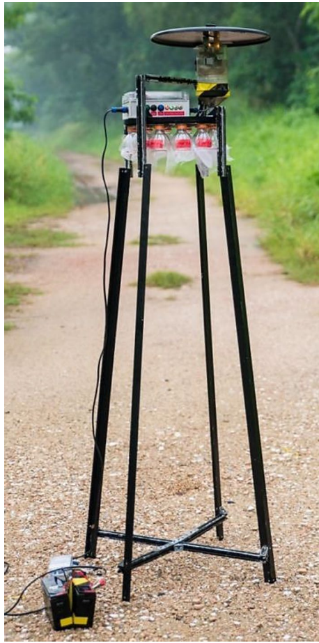
Fig. 2 Night Catcher is an in-house designed mosquito trap that enables trapping of mosquitoes at every hour. It was improvised from CDC light trap which uses incandescent light and dry ice (CO 2 ) as attractants
