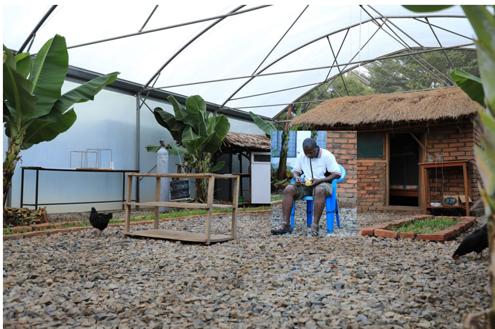
Fig. 1 Pictorial illustration of the semi-field chambers and experimental huts used inside the VectorSphere. The semi-field chamber was designed to mimic local mosquito ecosystems in rural villages in Ulanga and Kilombero district, south-eastern Tanzania. There were two experimental huts with brick walls and thatched roofs inside the chamber, which enabled assessment of indoor and outdoor mosquito-biting risk. Each evening, 500 hungry-female Anopheles arabiensis mosquitoes were released inside the chamber. Adult male volunteers sat in the peri-domestic space of each of the huts and collected mosquitoes attempting to bite them between 1800 and 2200 h, before going indoors to sleep under intact bed nets. CDC-light traps were used to catch mosquitoes attempting to bite the sleeper between 2200 and 0630 h the next morning. Photograph by Emmanuel Mwangi
