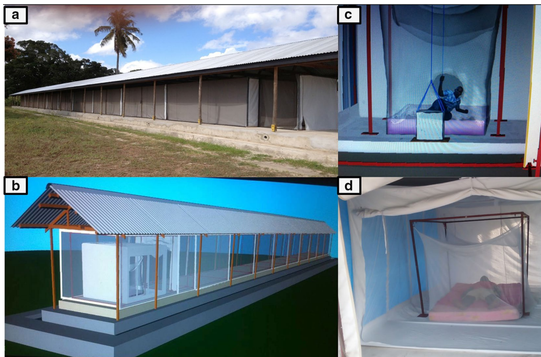
Fig. 1 The I-ACT. Ifakara Tunnel situated at Bagamoyo branch of IHI (a). Net covered tunnel divided into 10 individual compartments each containing netted cage 2 × 2 × 5 m (b). The volunteer releases mosquitoes by opening the lid of the holding boxes while beneath the tested net (c). A human volunteer sleeps underneath the ITN (d)
