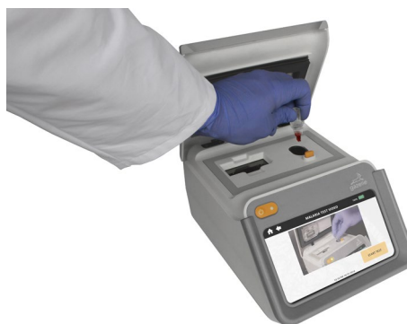
Fig. 1 The Gazelle™ Device. Battery-powered equipment that can run 200 tests independently. The diagnostic reader can store or upload patient data to a phone or computer for later storage in the Cloud. GPS location, useful for epidemiological studies, can also be saved
